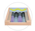
Alternating Pressure Gently changes loading across the surface (10-minute cycle).
