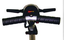
**LED Battery Indicator** is located on the top console of the Luggie scooter. As the battery is used, the LED indicator will move from green (fully charged) to red (low power).
