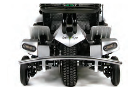
Quintell™ Self Centering Steering Advanced stability with agility plus defaults to straight line travel with minimal effort
