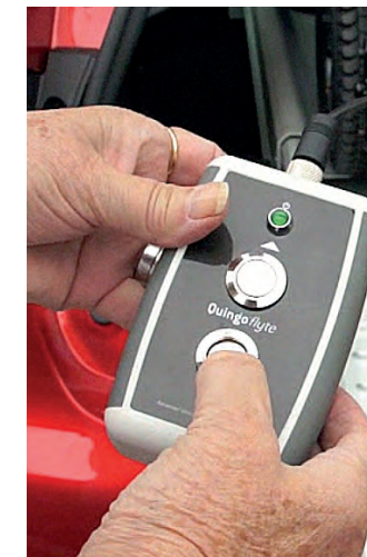
Quingo Flyte Remote Simple two button operation
